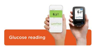
Each scan of the FreeStyle LibreLink app or reader over the sensor gives a current glucose reading, the last 8-hours of glucose history, and a trend arrow showing where your glucose is heading. The sensor can be scanned by your smartphone or reader through clothing with a thickness of up to 4cm.
